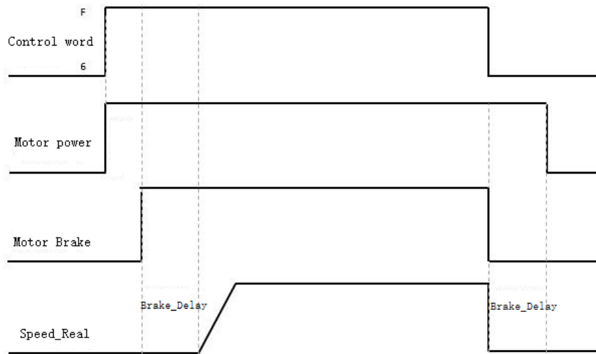
Figure 6-11 Motor holding brake sequence when quick stop mode is 0
