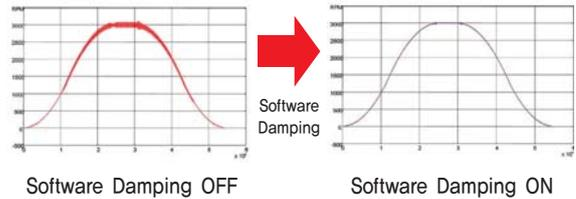
\*This is real measured speed that using 100000[pulse/rev] encoder.
