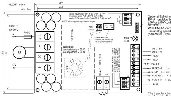
Optional braking resistor. Braking resistor needed in application where motor can supply energy back to supply Recom. values 0.5R @ 12V, 1R @ 24V Resistor power rating 50-200W, depends on solution
