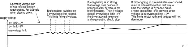
Freewheel options Normally motor poles is shorted in stop situation. and motor resist totating. With parameter can be set that driver disable power stage in stop and then the motor rotor run free. Also freewheel can beactivate during stop ramp (slowing down) then motor will not regenerate energy and not rise voltage.
