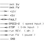
The input function in brackets is activated with parameter setting. speed input (param 5=0) speed input +dir. (param 5= 1)
