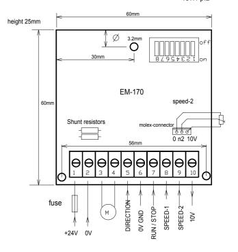
NOTE. With one shunt values will be halved current limit / A dip-switches 1-4 off on 0.2 000 0.3 00 0 ramp time / s 0.4 00 0.5 000 0 000 0.6 0.1 0.7 0 0 0.2 0.8 00 000 0.3 0.9 000 1 000 1.1 000 1.2 0\_00 1.3 00 1.4 dip-switch 8 00 0 1.5 "off" = decel. ramp OFF 000 1.7
