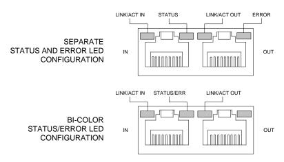
LINK/ACT IN and LINK/ACT OUT are used to drive the corresponding LINK IN and LINK OUT LEDs on a typical RJ-45 connector. The two STATUS/ERR pins are used to drive a bi-color Status LED or two separate single-color LEDs, depending on the user configuration (reference the DZEANTU Hardware Installation Manual for the recommended wiring diagram, available for download at <a href="https://www.a-m-c.com">www.a-m-c.com</a>). The LED Function Protocol tables below describe typical LED functionality.
