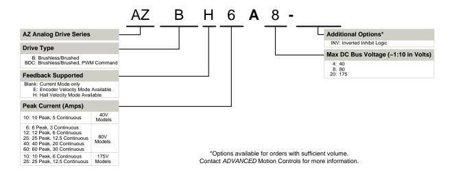
ADVANCED Motion Controls AZ series of servo drives are available in many configurations. Note that not all possible part number combinations are offered as standard drives. All models listed in the selection tables of the website are readily available, standard product offerings.
