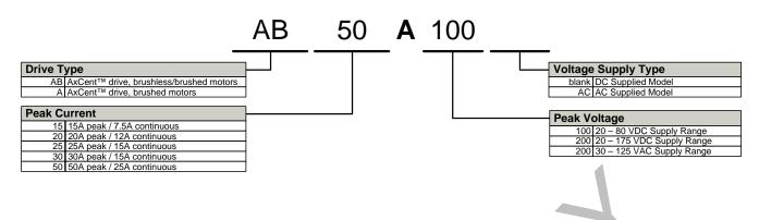
ADVANCED Motion Controls analog series of servo drives are available in many configurations. Note that not all possible part number combinations are offered as standard drives. All models listed in the selection tables of the website are readily available, standard product offerings.
